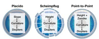
Figure 3: Each keratometry method - Placido, Scheimpflug, and Point-to-Point - is based on different principles
