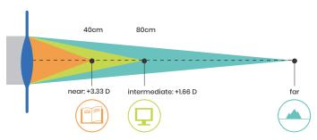
Figure 4: Trifocal IOLs have three distinct focal points for near, intermediate and far vision
