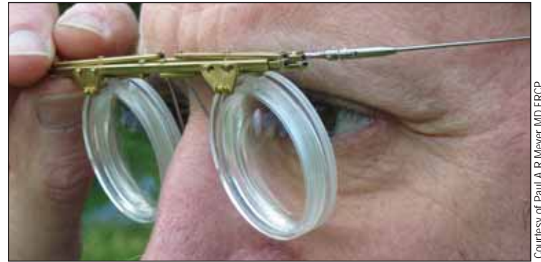
Manual alteration of the separation of the bars from any point adjusts the focal lengths of both lenses, identically.
